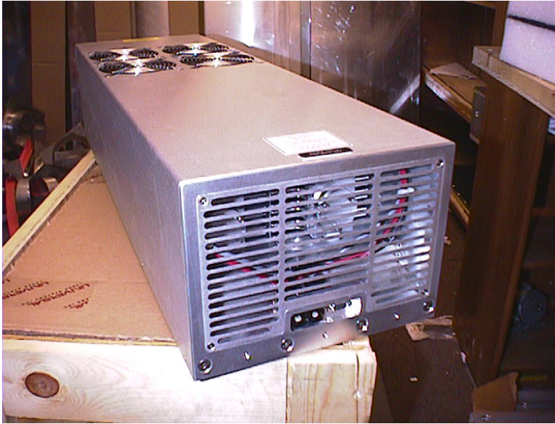
100 Watt Universal Air Cooled Tube (view from rear) Air exit grill may be removed for cleaning if required.
